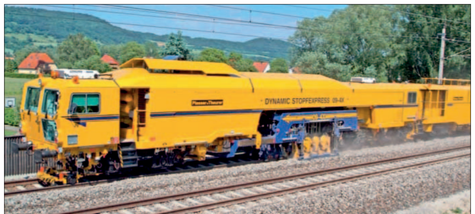
Figure 1: Continuous action four-sleeper tamping machine with integrated track stabilisation
