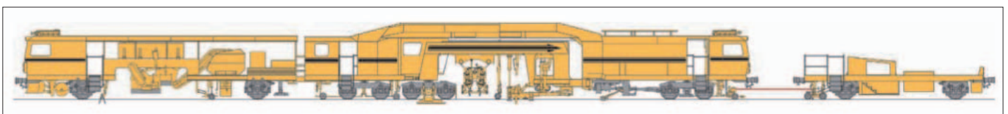
Figure 3: Continuous action switch tamping machine with measuring trolley (CAL-SAT)
