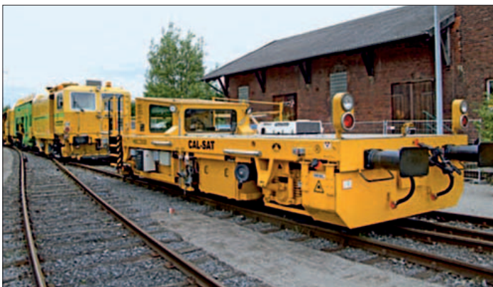
Figure 3: Continuous action switch tamping machine with measuring trolley (CAL-SAT)
