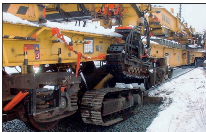
Fig. 5: Design of the "PK1" gantry crane for the WM 500 series (left and right)
