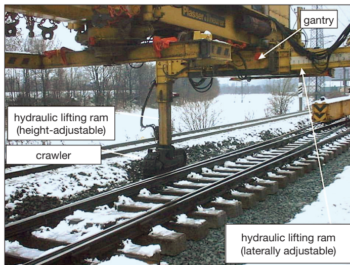
Fig. 6: The "WRW" as the transport vehicle for the "PK1"
