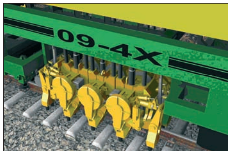
Fig. 7a: Operation as a continuous-action four-sleeper tamping machine
