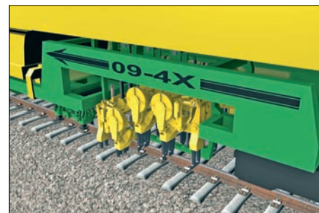
Fig. 7c: Operation as a continuous-action single-sleeper tamping machine
