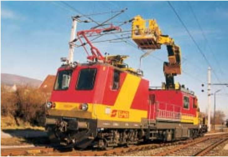
Fig. 6: The MTW 100.083/1 for both constructing and maintaining catenaries
