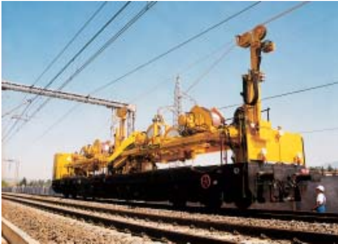
Fig. 4: Catenary-replacement machine with a directional telescopic column
