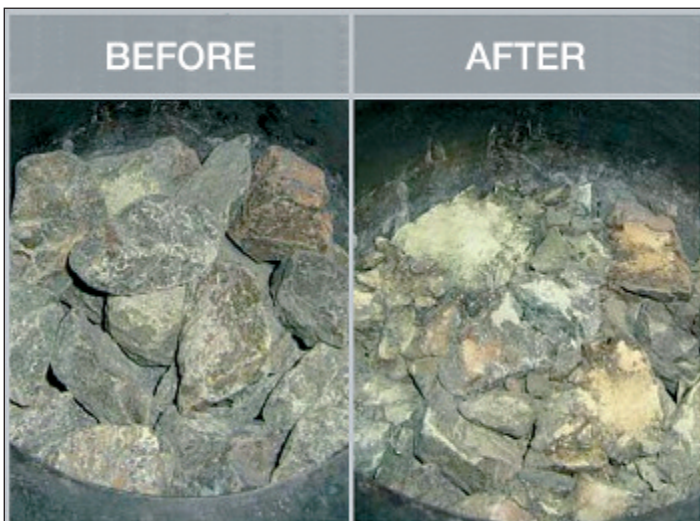
Above: Figure 4: Stone sample before and after an impact fragmentation test as per [12] (Source: ÖBB).
