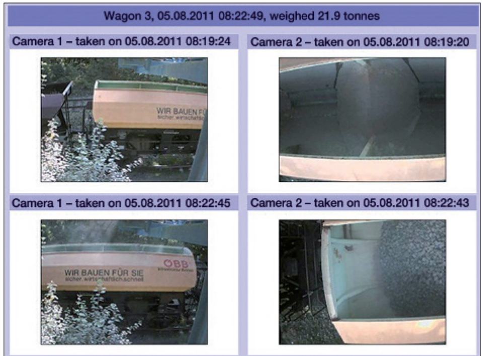
Above: Figure 9: Images from the automatic loading control of an ÖBB track ballast supplier showing the video surveillance at various stages of loading - documentation of wagon number, wagon empty, loading process and load weight. (Source: ÖBB).
