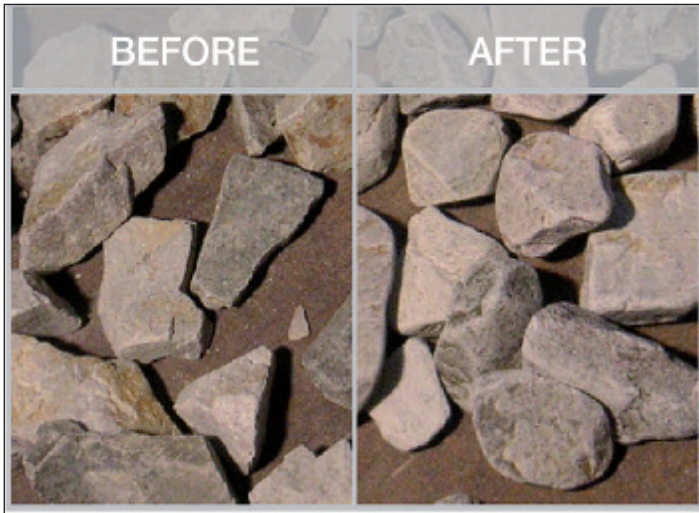
Left: Figure 6: Stone sample before and after a Micro-Deval test as per [13] (Source: ÖBB).
