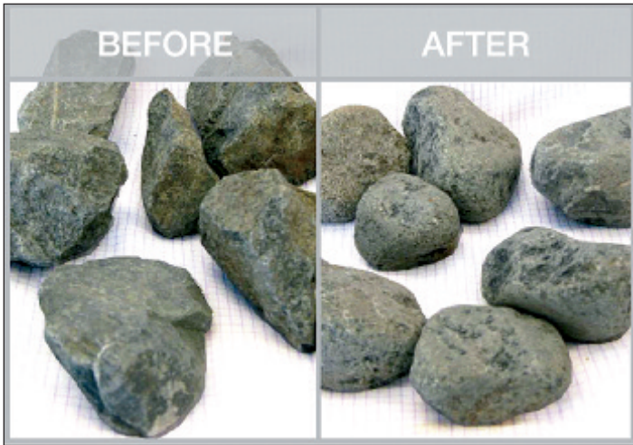
Above: Figure 2: Stone sample before and after a Los Angeles test as per [12] (Source: ÖBB).
