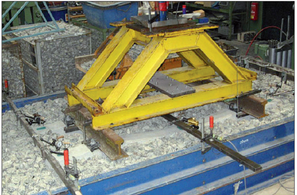
Above: Figure 15: Test rig during the fatigue level test. (Source: ÖBB).
