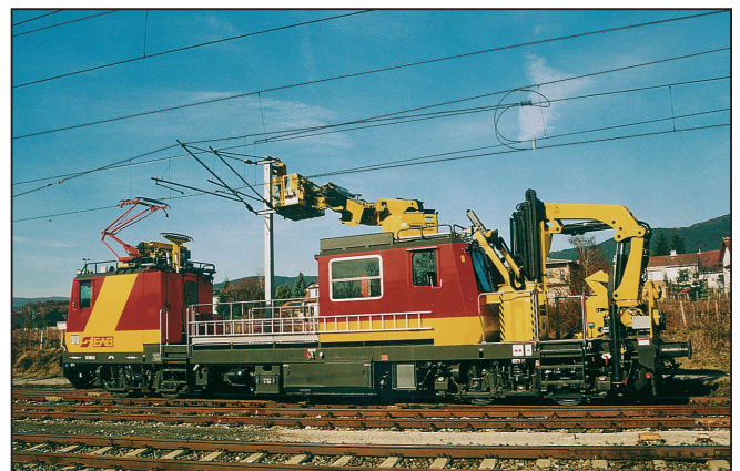
Fig. 5: Motor tower car - MTW (above) with contact wire and carrying cable holding device (left) and measuring pantograph with proximity sensors (below)
