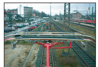
Fig. 5: Motor tower car - MTW (above) with contact wire and carrying cable holding device (left) and measuring pantograph with proximity sensors (below)
