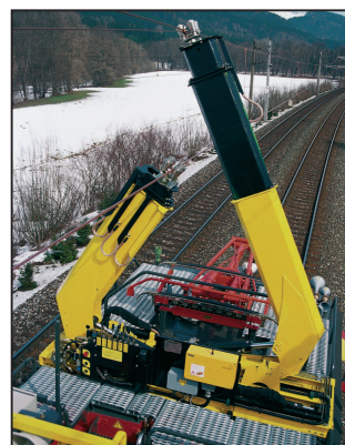
Fig. 5: Motor tower car - MTW (above) with contact wire and carrying cable holding device (left) and measuring pantograph with proximity sensors (below)
