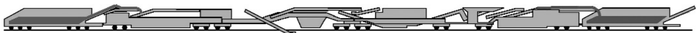
Fig. 13: Ballast cleaning machine, together with material conveyor and hopper (MFS) unit for the supply of new ballast and the transport of spoil
