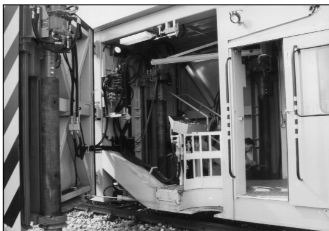
Fig. 1: The UUM subsoil probing machine, featuring three boring units for taking boring cores from the track
