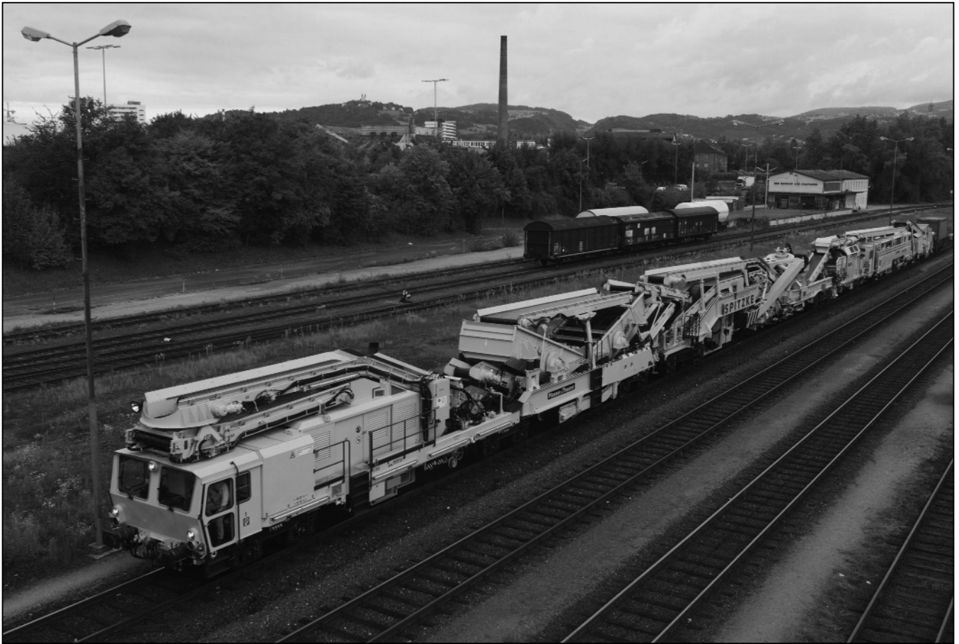
Fig. 14: The Plasser & Theurer RM 900 S ballast cleaning machine, which features a total mass of 345 t and a construction length of more than 100 m
