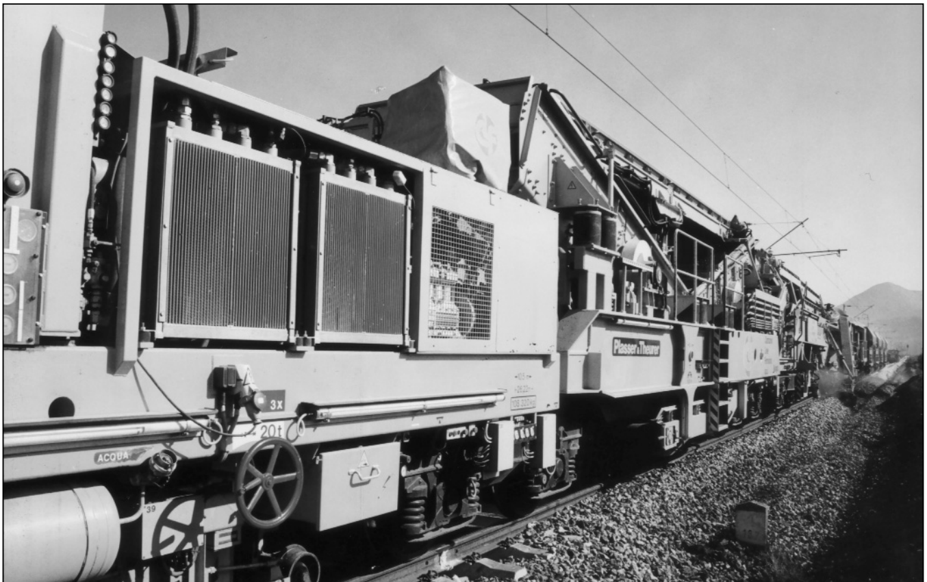
Fig. 8: Double screening unit of the Plasser & Theurer RM 860 ballast cleaning machine
