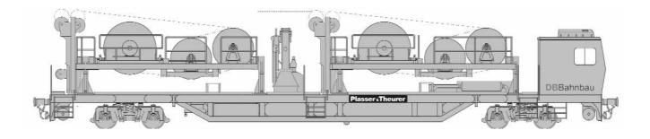
Fig. 2: Diagram of the FUM 100.128 catenary renewal machine, which features a driver's cab, two tilting winch units and underfloor drive units
