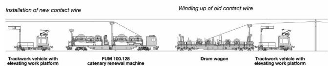
Fig. 5: Exchange of contact wire only
