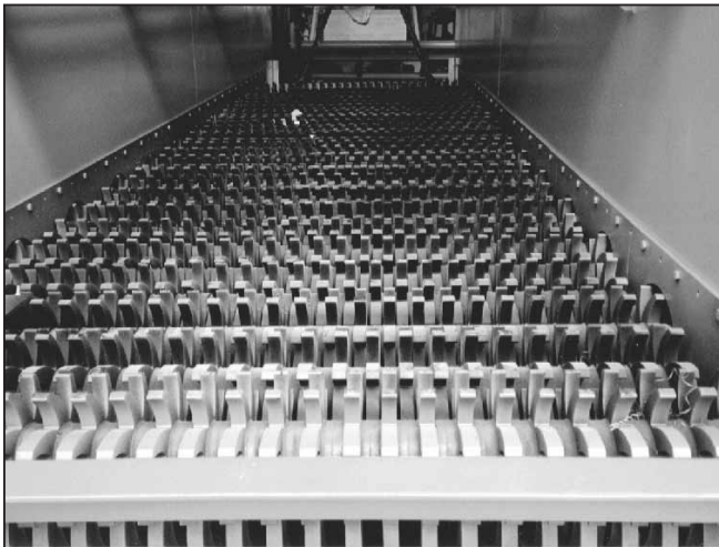
Fig. 10: Star screen (system Wiebe)
