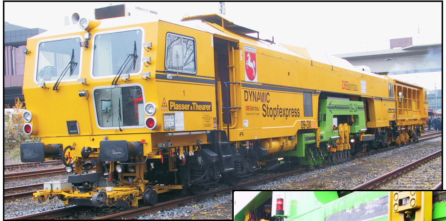
The Dynamic Tamping Express consists of a three-sleeper tamper coupled to a dynamic track stabiliser.
