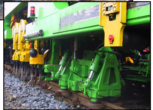
The Dynamic Tamping Express consists of a three-sleeper tamper coupled to a dynamic track stabiliser.
