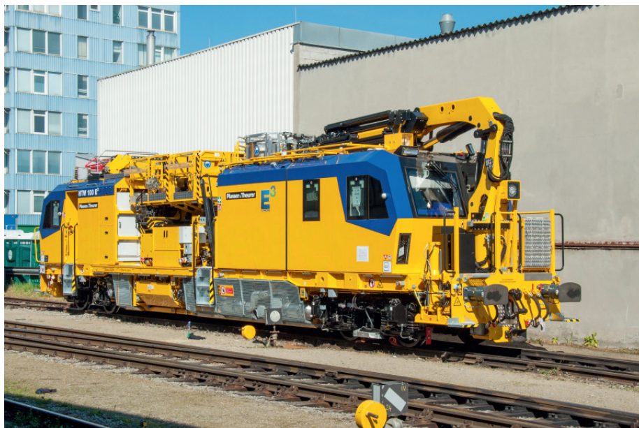
FIG 2: The new HTW 100 E 3 catenary maintenance machine is equipped with batteries for electric working operation
