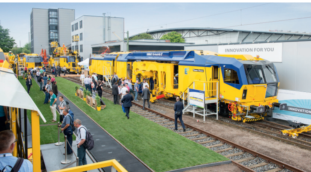
FIG 1: The new Unimat 09-4x4/4S E 3 universal tamping machine has been designed for fully electric or diesel-electric operation
