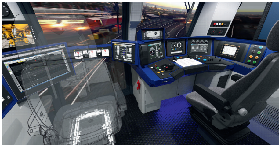
FIG 7: Digital control elements and touch screens enable ergonomic operation and shape the cabin design on the latest generation of track maintenance machines
