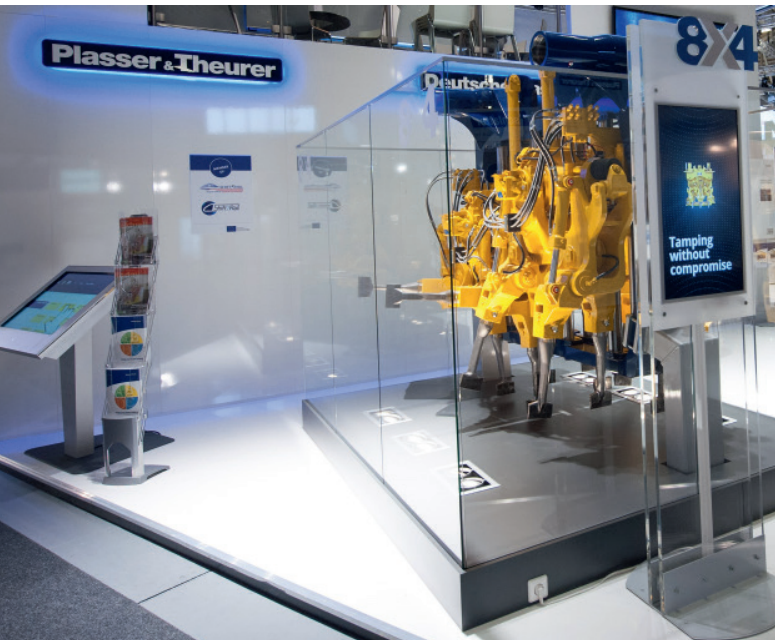
FIG 3: The new 8x4 tamping unit
