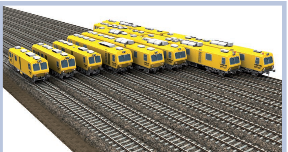
Fig. 3: Plasser & Theurer offers a standardised selection of track recording cars
