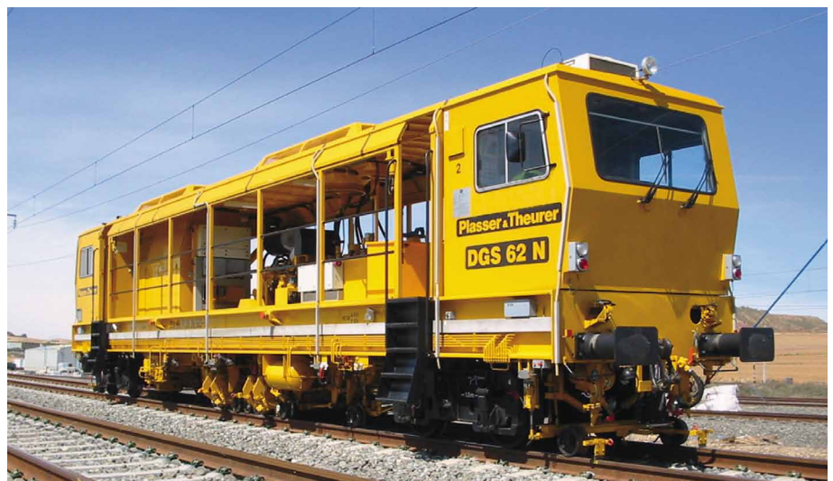
Fig. 7: The four-axle DTS 62 N standard design
