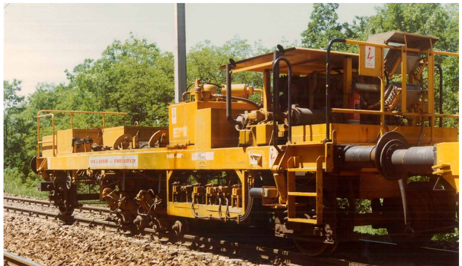
Fig. 4: The first Dynamic Track Stabiliser, designed as tamper trailer
