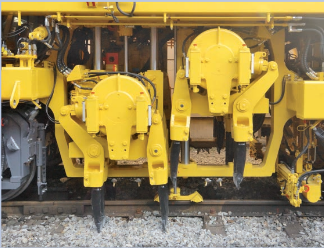
Fig. 6: 1 or 2-sleeper tamping at the push of a button – 09-2X/SD (factory photo, without sound protection panels)
