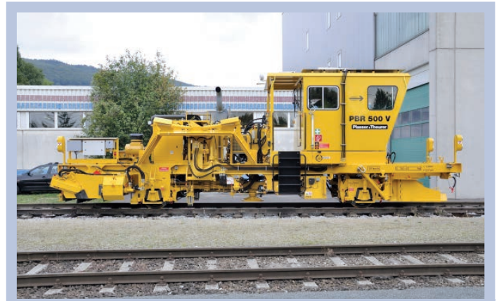
Fig. 3: Easy ballast regulating – PBR 500 V (factory photo)
