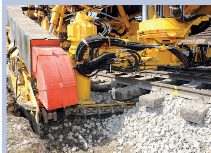
Fig. 9: Excavating unit of the URM 700
