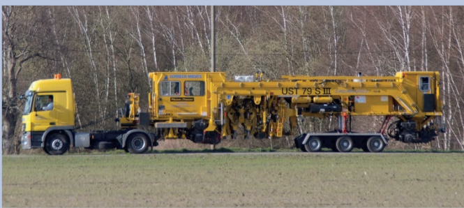
Fig. 7: By road to the worksite – UST 79 S tamping machine
