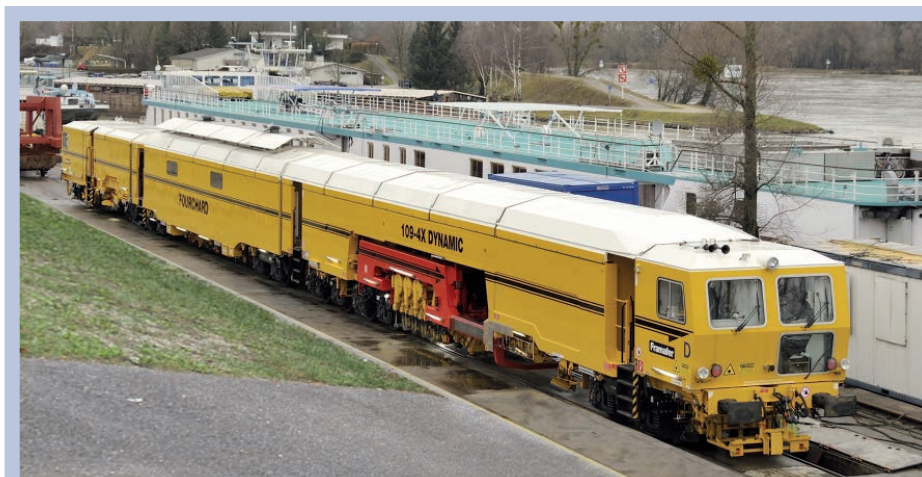
Fig. 1: The fastest track tamping machine in the world – 109-4X Dynamic Tamping Express (factory photo) (source of all figures: Plasser & Theurer)
