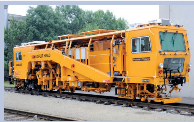
Fig. 2: Tamping machine with split-head technology – Plasser 08-16 SH (factory photo)
